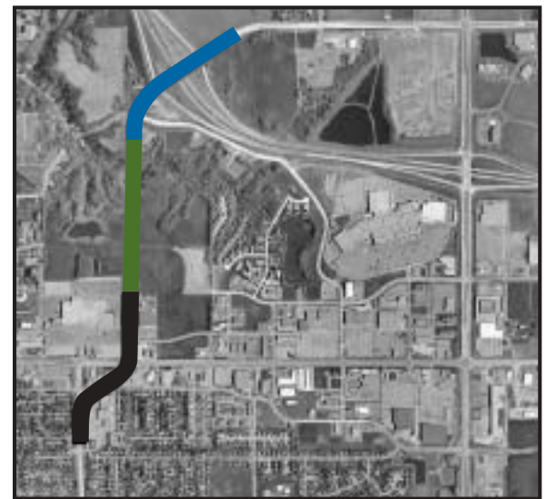
The second stage of the Victory Drive Extension, which includes a bridge across Thompson Ravine, will run south to Holly Lane on the east side of Madison East Shopping Center.
