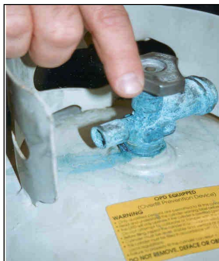
Blue valve means danger!
